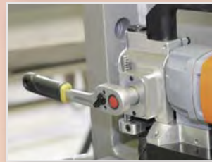
Fed using ratchet leveler, reversible for right- and left-handed operation
